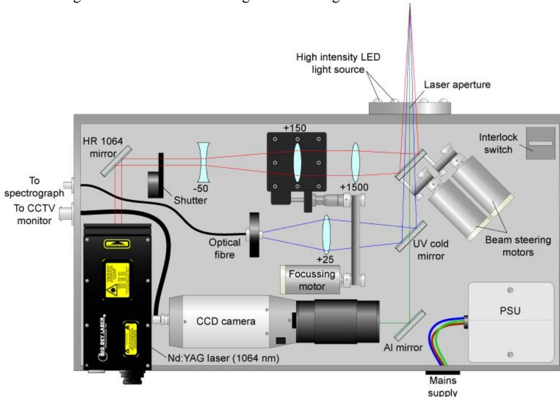
**Schematic diagram of the laser module of the telescope LIBS instrument used to identify reinforcing bars and cooling water tubes within the concrete pressure vessel of a Magnox reactor**
