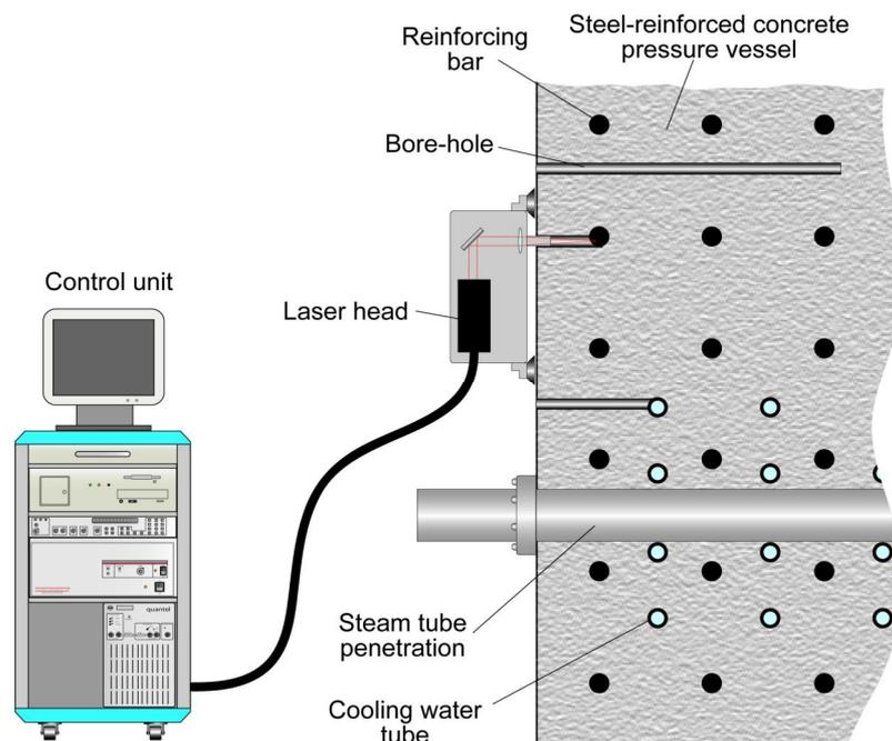
**Schematic diagram illustrating the method of deployment of the LIBS instrument**
