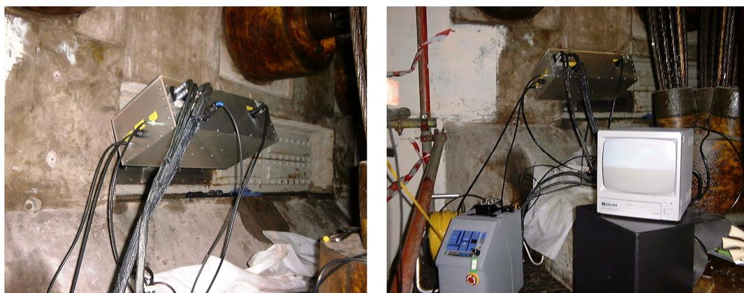
**Images of the LIBS instrument being deployed at the reinforced concrete pressure vessel wall of a Magnox reactor**
