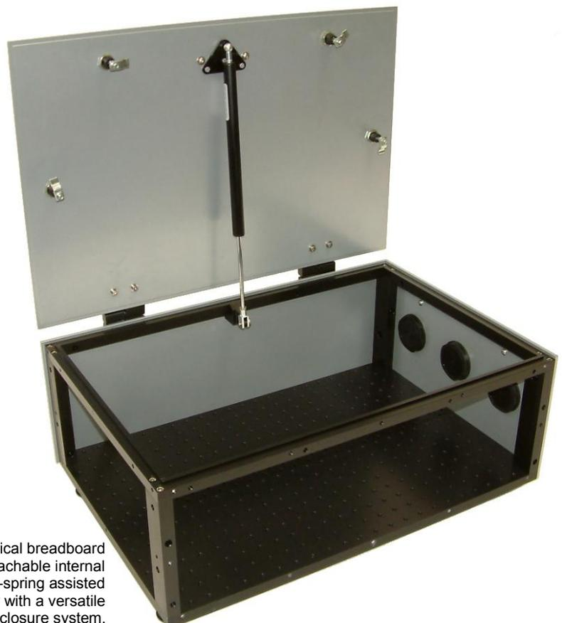
The combination of a heavy-duty optical breadboard base, removable side panels, detachable internal support frame components and a gas-spring assisted hinged lid provides the optical engineer with a versatile and modular enclosure system.
