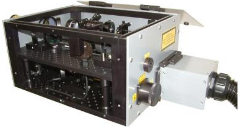
Customised System 400 enclosure - an example of what is possible; a prototype laser spark analyser instrument designed and manufactured by Applied Photonics Ltd.
