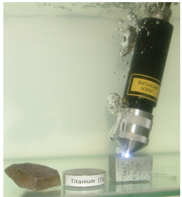
Sample materials submerged in water being analysed by the LIBS instrument
