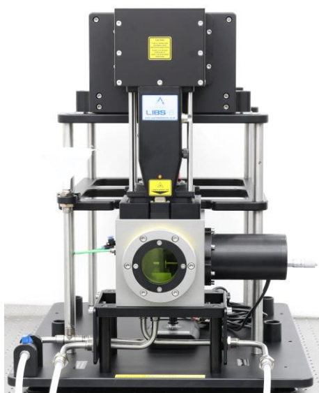
LIBS-6 module with laser head and adaptor platform using one of our modular SC-LQ2 sample chambers.
