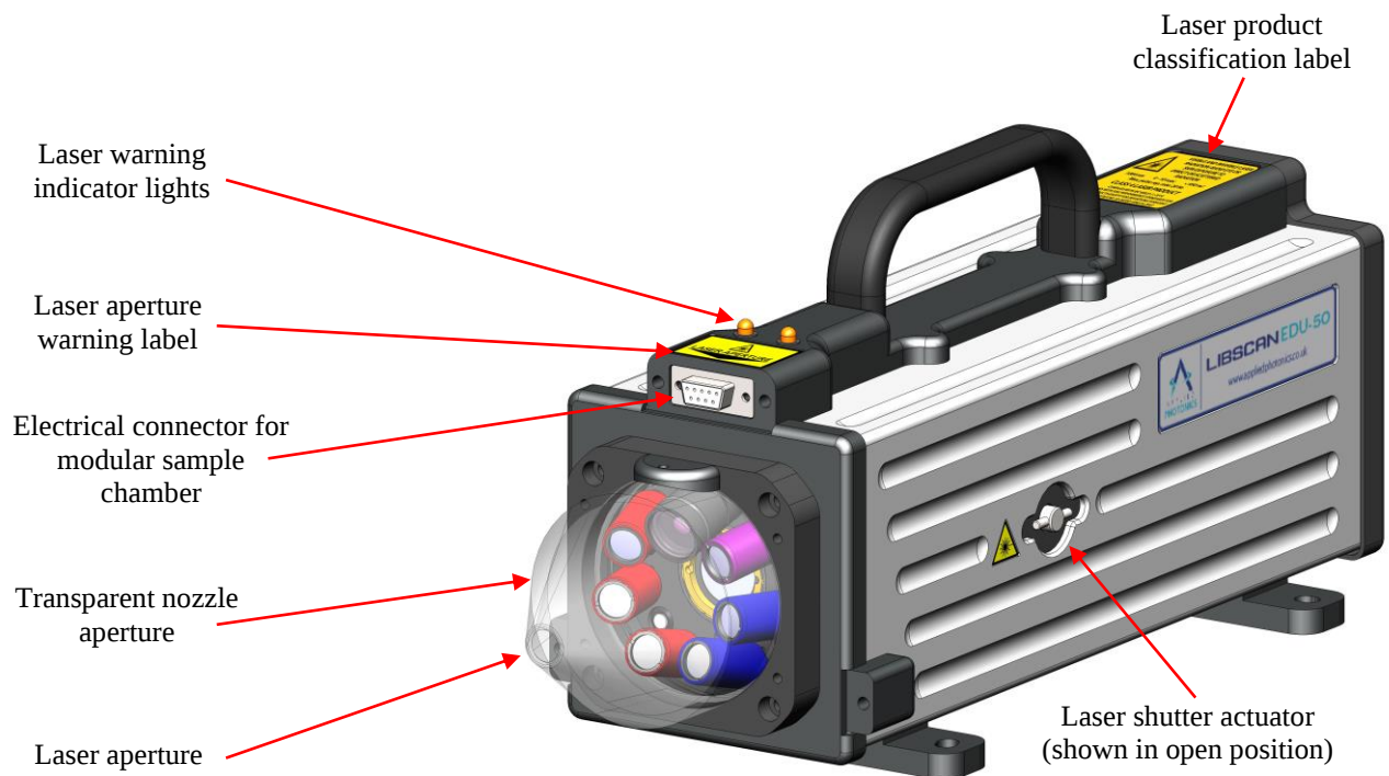
CAD image of LIBSCAN EDU-50 head showing location of laser warning indicator light, laser aperture, laser warning labels, laser shutter actuator and the electrical connector interface for the modular sample chamber
