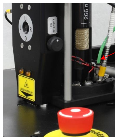
Image of LIBS-6 module showing pneumatic tube connected to “push fit” connector
